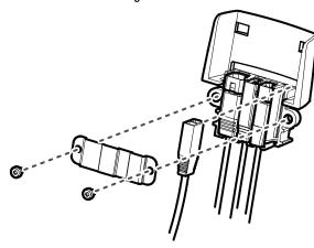
8. Place the cable collector assembly into the back of the control head. Cable connectors and cable sockets are keyed to prevent reverse installation, so be careful not to force the connectors into the wrong sockets.
